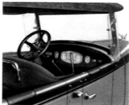
Note the extremely well designed and attractive instrument panel. Every instrument placed where it can be seen, every manual control at the finger tip.
