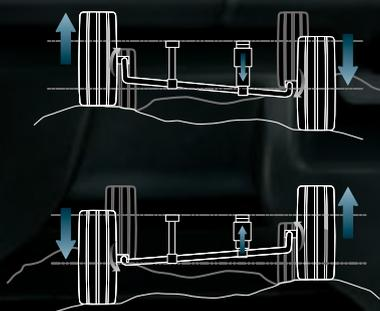
Stabilizer bars help minimize body roll on the road, but can be a hindrance on uneven trails by preventing tires from maintaining contact with the ground. To counter this, the Kinetic Dynamic Suspension System uses hydraulic cylinders to adjust the bars in off-road conditions. When
