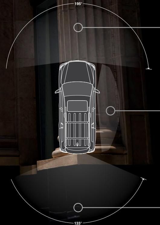
The available Wide-view Front and Side Monitor system<sup>11</sup> uses a grille-mounted camera to help enhance visibility of what's just around the corner.
