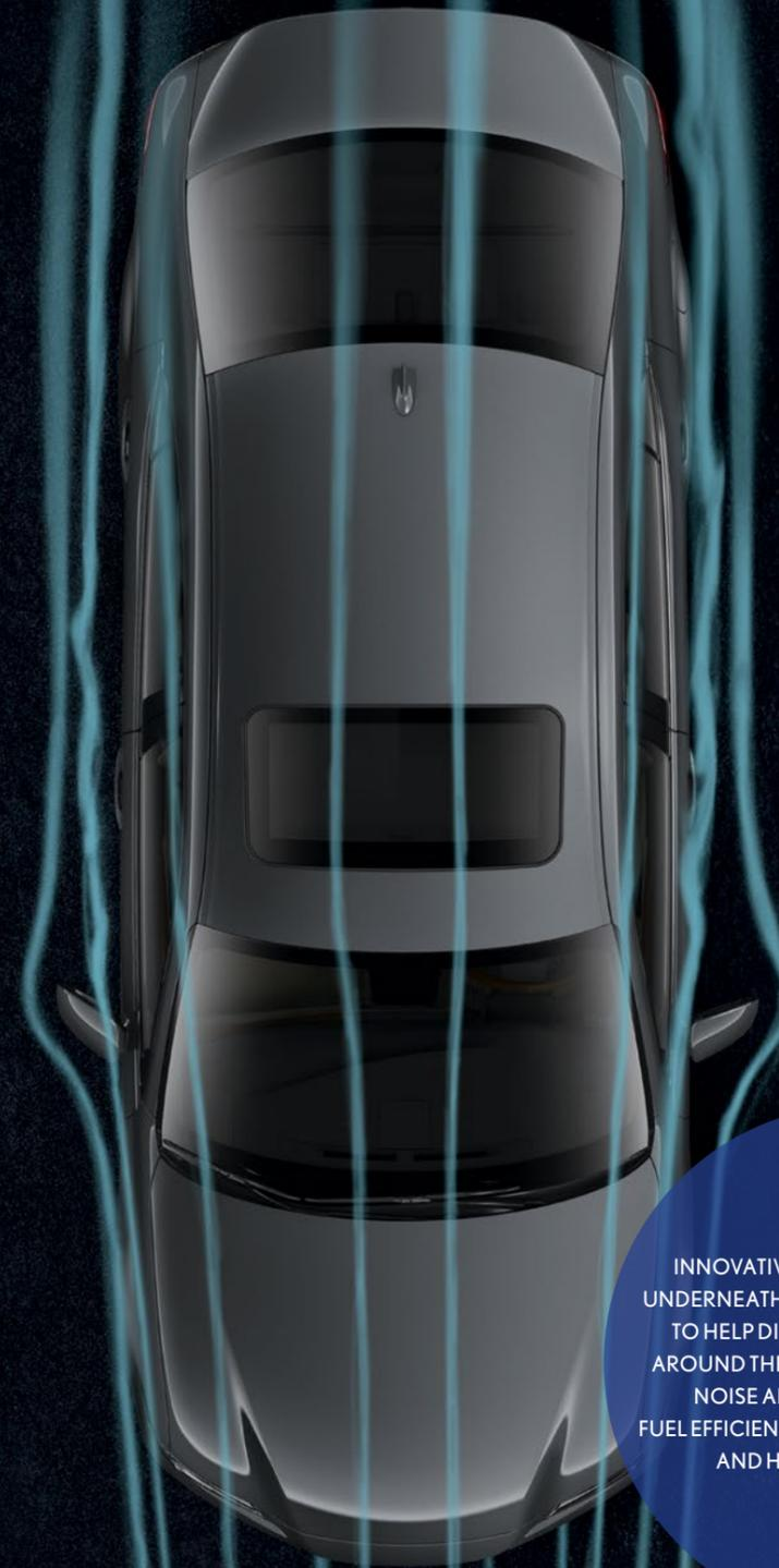
INNOVATIVE MEASURES WERE TAKEN UNDERNEATH AND ON THE SIDES OF THE ES TO HELP DIRECT AIRFLOW SMOOTHLY AROUND THE BODY, HELPING TO REDUCE NOISE AND VIBRATION, IMPROVE FUEL EFFICIENCY, AND ENHANCE HANDLING AND HIGH-SPEED CONTROL.
