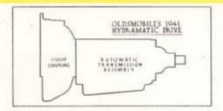
Oldsmobile's Hydra-Matic Drive is self-contained and requires no extra attachments. It replaces both the conventional clutch and the transmission.
