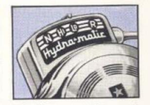
"Lo" from "Hi" instantly. At speeds above 40 M.P.H., a special "cut out" automatically takes the "Lo" range out of operation since it can serve no purpose at the higher speeds.
