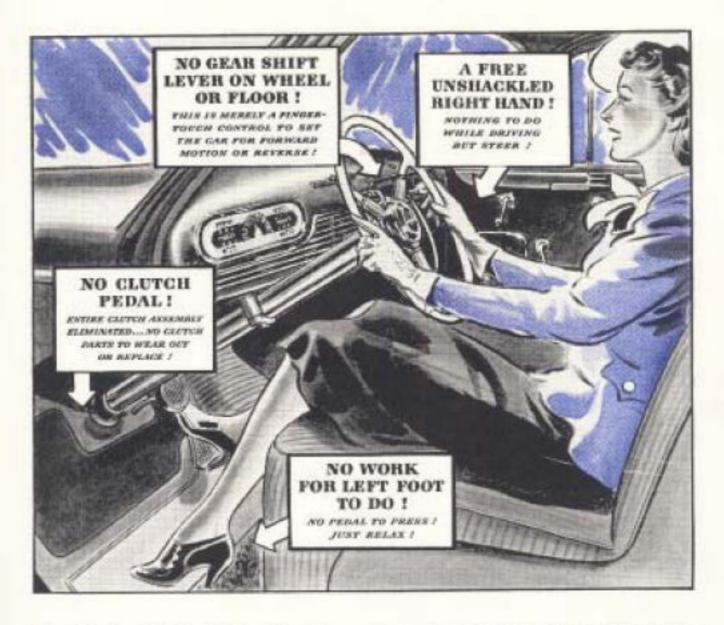
The Hydra-Matic Drive directioncontrol lever, conveniently located just below the steering wheel, is in no sense a gear shifter, as all action is automatic. The position farthest to the left is neutral, and is used when parking. The next position, to the right, is "Hi," and is used for all normal driving. Once in "Hi," it is not necessary to move the lever for starting, stopping or accelerating. The third position is marked "Lo." This speed
