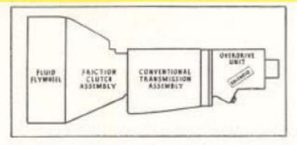
The drive diagrammed above does not eliminate any unit of the old-fashioned transmission system. It merely superimposes two extra accessory units upon the conventional drive — the fluid flywheel coupling and an over-drive.
