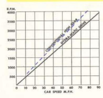
Wear and tear on bearings, pistons, cylinder walls and all reciprocating parts is materially lessened by slower engine speeds. There are no clutch facings and clutch parts to be replaced. The slow-moving propeller shaft and universal joints are less subject to shock and wear. Smoother starts and stops reduce tire scuffing and result in longer tire life.
