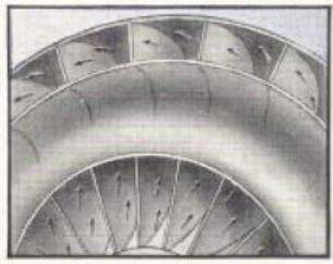
However, the liquid coupling offers little or no advantage in car operation unless it is combined with an automatic transmission.
