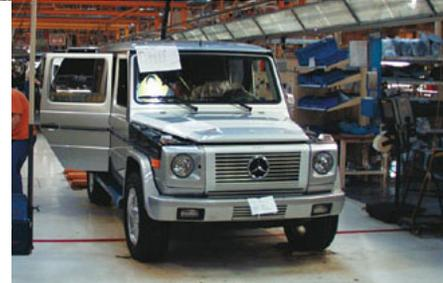
While workers are busy installing the engine, drivetrain, suspension and various other components onto the frame, an artisan upstairs expertly weaves hundreds of feet of wires into a single vehicle's wiring harness. Once this harness is installed in the vehicle, many of the body cavities are filled with more corrosion-resisting wax.
