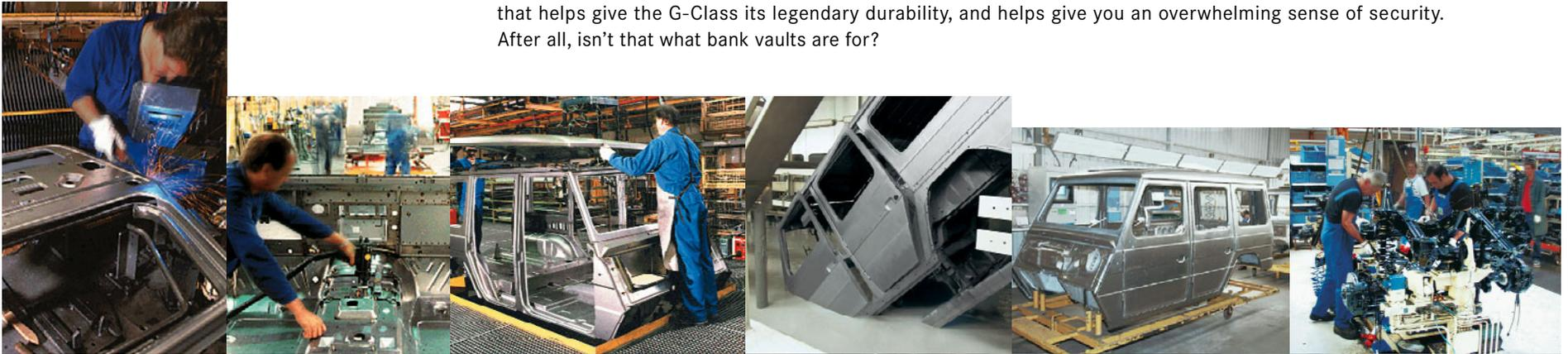
Life for the G-Class begins in the inspired hands of its craftsmen. In fact, from the very first weld, each craftsman signs off on his or her part of the process. An extremely rigid steel frame is constructed using fully boxed longitudinal rails and six tubular crossmembers to further enhance torsional stiffness.
