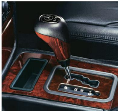
Controlling all that power is a driver-adaptive electronic 5-speed automatic transmission featuring the manual-style operation of Touch Shift. Nudge the shift lever to the left of Drive to downshift, or to the right to allow the transmission to shift into a higher gear. Or hold the lever to the left for a second and the transmission automatically chooses the ideal passing gear. Now you're in command – of your G-Class and the road ahead.
