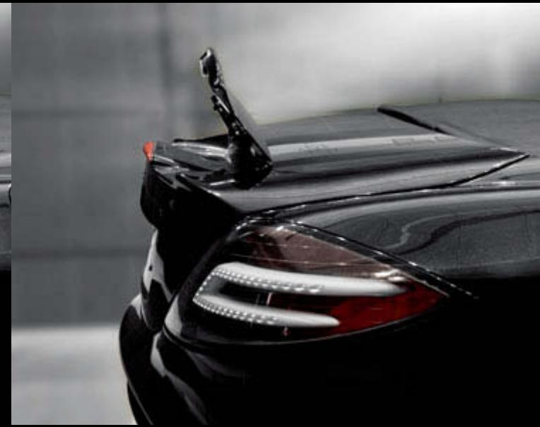
Automatically raised to 65 degrees in the event of abrupt braking
