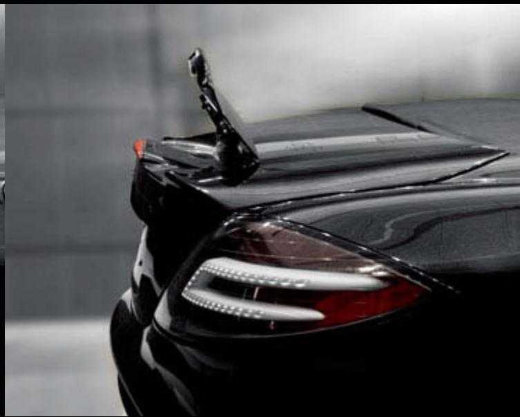
Automatically raised to 65 degrees in the event of abrupt braking
