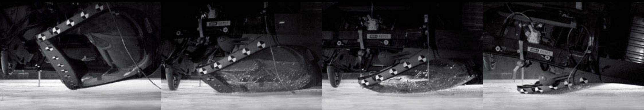
The SLR Roadster undergoing a roof-drop test: the newly developed hybrid A-pillar with steel core can support the whole vehicle weight
