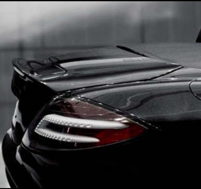
The AIRBRAKE in zero position
