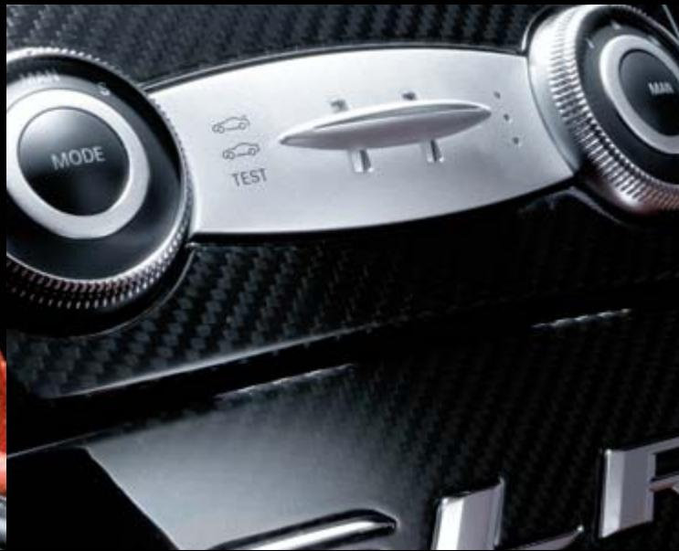
Switches for transmission modes, AIRBRAKE and gear-change speed
