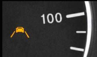
**Lane Keeping Assist**<sup>7</sup> provides the driver with audible and visible warnings if the vehicle leaves its lane unintentionally. A camera in the windshield monitors the road ahead, detecting when you may veer away from lane markings.
