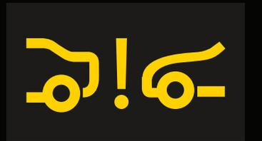
**COLLISION PREVENTION ASSIST**<sup>6</sup> is a radar-based proximity warning system that issues visual and audible warnings when vehicles traveling ahead come within a potentially dangerous distance. In emergency situations, boosted braking pressure levels assist automatically to help prevent rear-end collisions.
