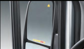
**Blind Spot Assist**<sup>5</sup> helps the driver avoid accidents by giving visible warnings when it detects vehicles in the blind spot.
