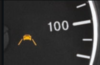
**Lane Keeping Assist<sup>6</sup>** provides the driver audible and visible warnings if the vehicle leaves its lane unintentionally. A camera in the windshield monitors the road ahead, detecting when you may veer away from lane markings.
