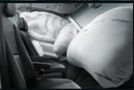
The Sprinter features height-adjustable 3-point seat belts, two-way headrests and front airbags to keep drivers—and passengers—safe.<sup>10</sup> Optional window and thorax airbags<sup>10</sup> offer even greater protection.
