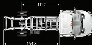
Choose between two wheelbases (144 inches and 170 inches) both with GVWRs of 11,030 pounds, and build the Sprinter Cab Chassis that works best for you.
