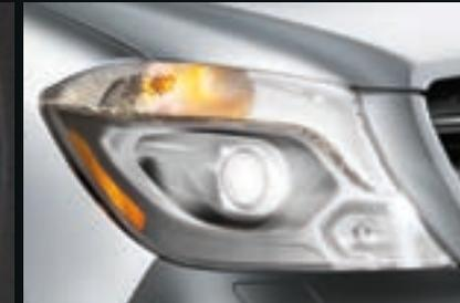
**Highbeam Assist** utilizes a camera located on the inside of the windshield to monitor traffic ahead. When activated, it controls the headlight main beam to provide the best possible road illumination.
