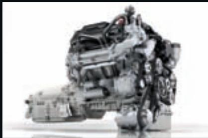
The optional 3.0-liter V6 turbo diesel engine is a proven powertrain that offers powerful acceleration, 325 lb-ft of torque combined with a smooth 5-speed transmission.
