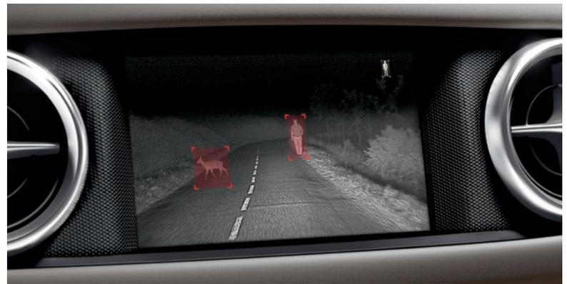
**Nighttime enlightenment.** Available Night View Assist PLUS<sup>6</sup> projects infrared beams that are invisible to the human eye, and reads them with a special camera. It displays a supplemental view of the road on the in-dash COMAND<sup>®</sup> screen, highlighting pedestrians and some animals. A focused flash of the headlights helps alert pedestrians. You can also set the display to turn on only when it senses a pedestrian or animal.<sup>10</sup>
