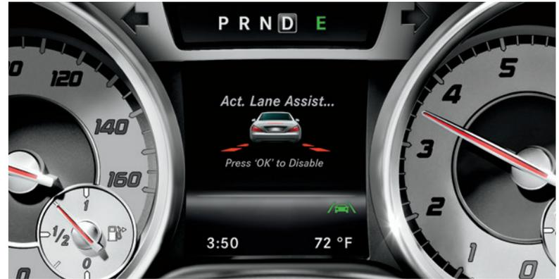
**Multilane multitasker.** Available Active Lane Keeping Assist<sup>6</sup> uses a camera to monitor the car's position relative to visible lane markings. If you start to drift out of your lane without using a turn signal, it can alert you by vibrating the steering wheel. If you disregard the system's alerts, its advanced active technology can also gently apply the brakes to individual wheels, to help draw the vehicle back into its original lane.<sup>9</sup>
