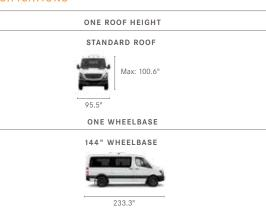
All measurements in inches. All width measurements include mirrors. See page 45 for a complete listing of models and specifications.
