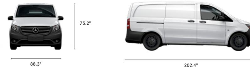
All measurements in inches. All width measurements include mirrors. See page 29 for a complete listing of models and specifications.
