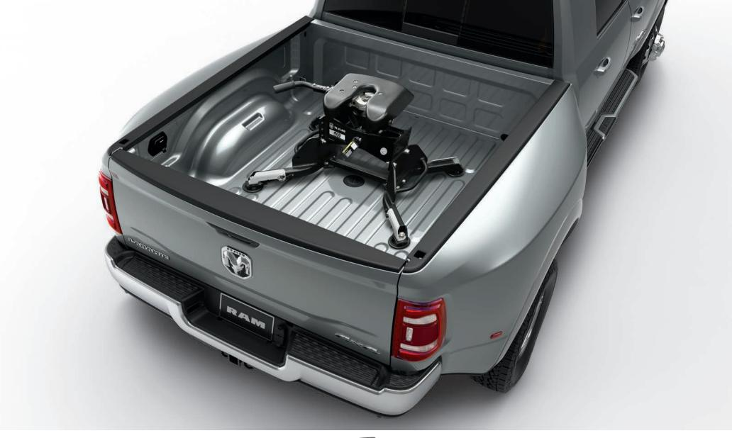
A MAJOR INCREASE in towing capacity comes from an upgrade to the fully integrated rear-axle crossmember structure on all frames. The available fifth-wheel hitch mounting hardware is integrated into the production box floor—and includes fifth-wheel pucks.
