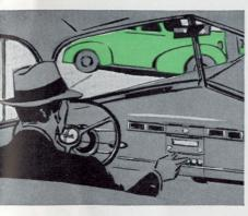
Hudson Unitized Auto Radios are especially designed, engineered and built for Hudson cars. A single unit, they fit between the instrument panel and the dash-with the control head and speaker integral with the sets, eliminating all cables, and thus not taking away from leg room space. AUTOMATIC PUSH BUT-
