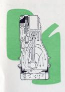
generous streams of oil are driven to working parts by the over-sized pump. One stream goes to the front of the motor; the other to the rear. This assures ample, efficient lubrication on hills as well as on level roads. The labyrinthian system then cools the oil before it is filtered and recirculated. Most important is the fact that the flow of oil in your Hudson increases in direct proportion to the speed of your motor. No other lubrication offers these important advantages.
