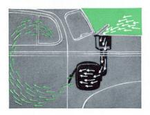
Hudson Weather-Master Fresh Air and Heat Control, which includes an air filter and fits up snugly under the cowl ventilator.
