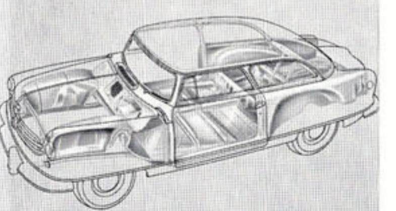
**Airflyte Construction** stays new years longer because it's a single, welded unit—twice as rigid as ordinary separate body and frame construction. It is free of the usual squeaks and rattles.
