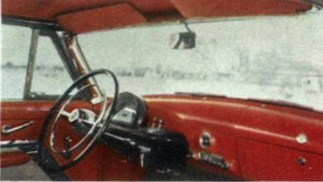
Mercury's Interceptor instrument panel brings instruments and controls closer for practical, easier use. All instruments are arranged in convenient cluster for quick reading recognition. All controls are grouped directly before you within easy reach for finger-tip operation.
