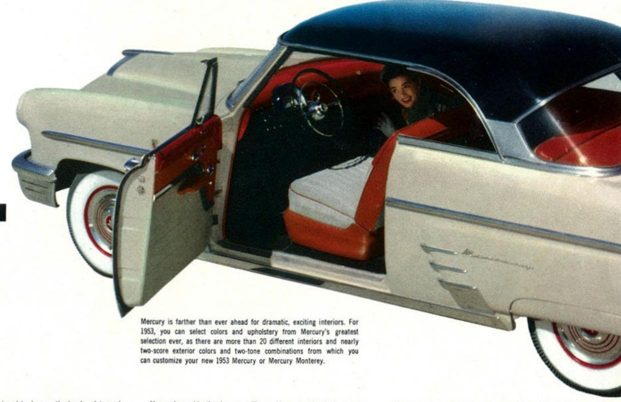
Mercury introduces the two-stop door as a feature of Unified Design. You can stop front doors either half-way or full-open. It's a great convenience in your garage, driveway, or other close places. On Mercury, all doors are front-hinged to open against the windstream, for extra safety.
