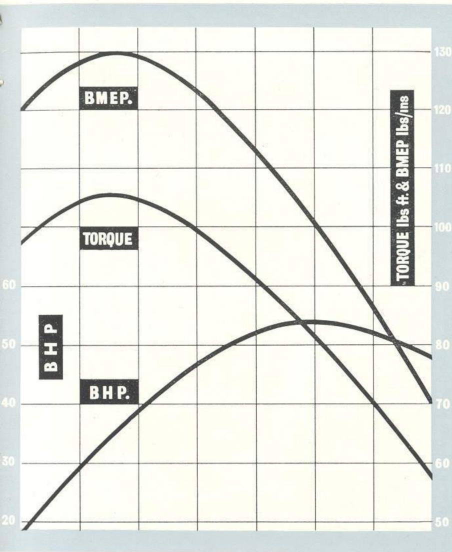
As shown on the graph above, the Land-Rover engine develops 52 b.h.p. at 4,000 r.p.m., while the excellent torque figure of 101 lb./ft. at 1,500 r.p.m. represents outstanding pulling power at low revs. The cubic capacity of the unit is 1,997 c.c. and its compression ratio is 6.9 to 1.
