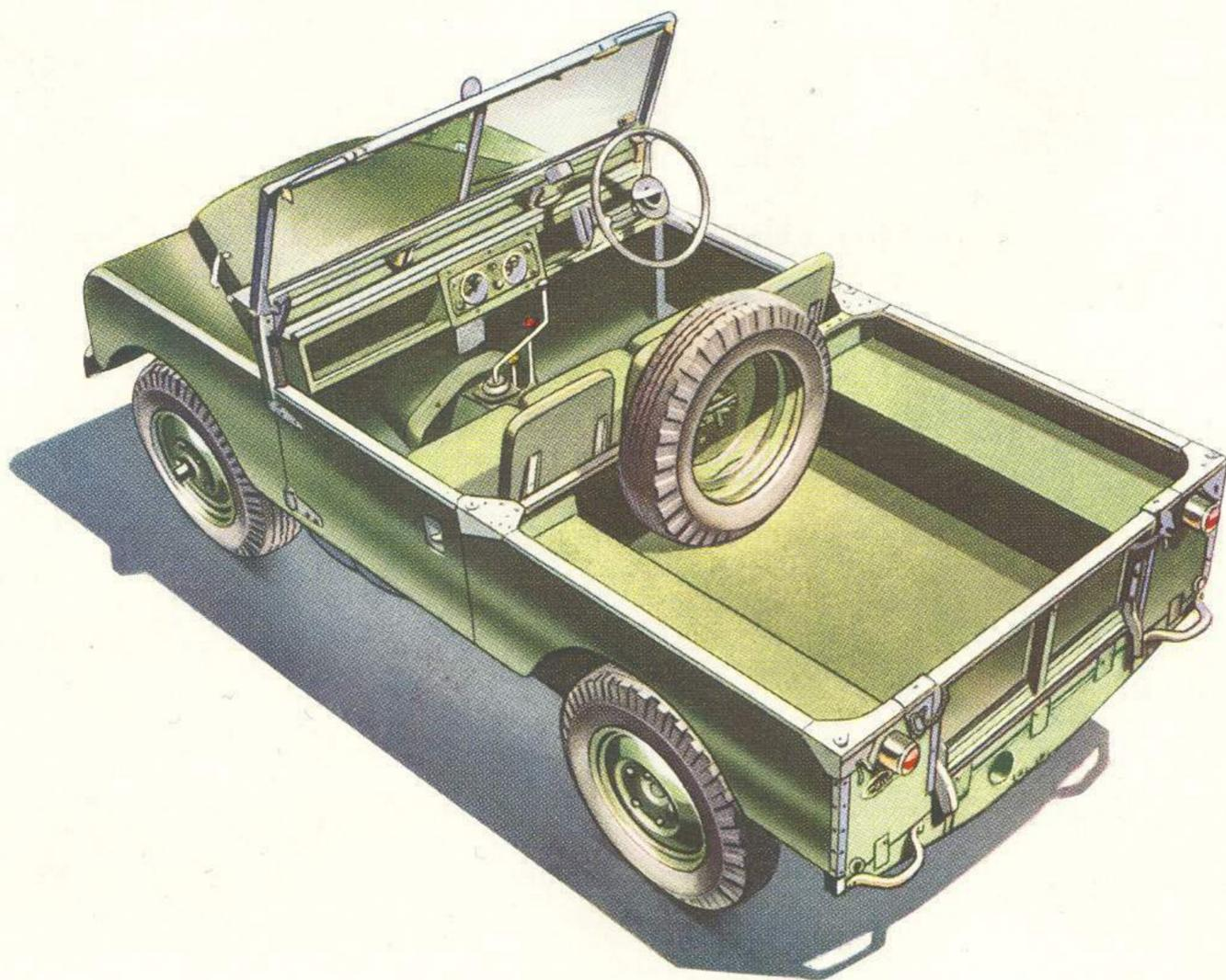
The 86 in. wheelbase, four-wheel drive Land-Rover is the general factotum of the range, providing the sort of go-anywhere transport that is needed on farms, ranches, estates and indeed in any situation where versatility and cross-country mobility are required. It can operate as a completely open vehicle or be fully enclosed by the weather-proof canvas hood. In either event the body provides excellent accommodation for three people and loads of up to 1,000 lb. (454 kg.).
