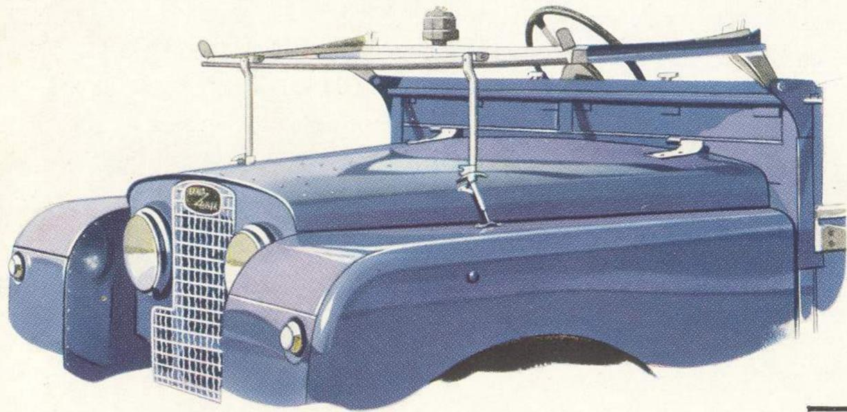
When required, the windscreen can be folded forward. It is held in this position by supports which are secured by the bonnet catch on each side.
