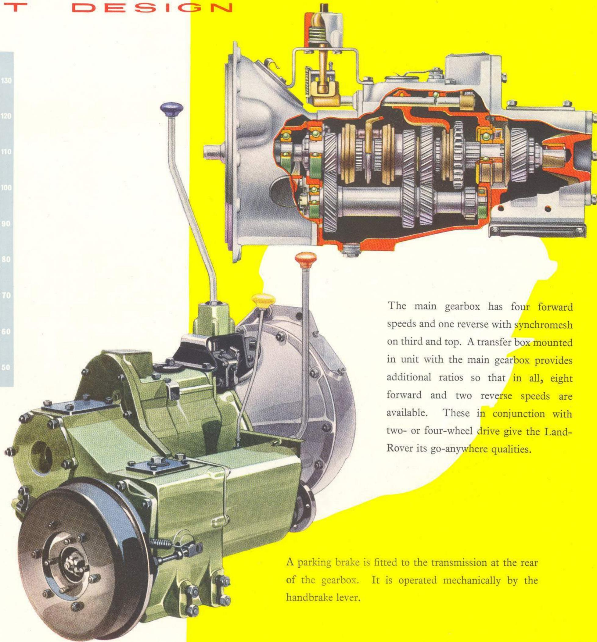
The main gearbox has four forward speeds and one reverse with synchromesh on third and top. A transfer box mounted in unit with the main gearbox provides additional ratios so that in all, eight forward and two reverse speeds are available. These in conjunction with two- or four-wheel drive give the Land-Rover its go-anywhere qualities.
