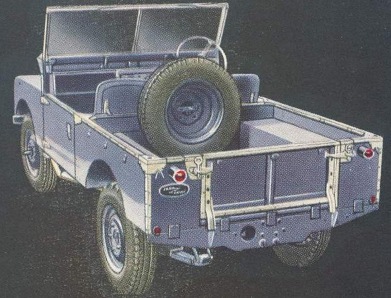
The detachable hard-top has a lift-up type of door at the rear. With the vehicle tailboard lowered ample loading facilities are afforded.
