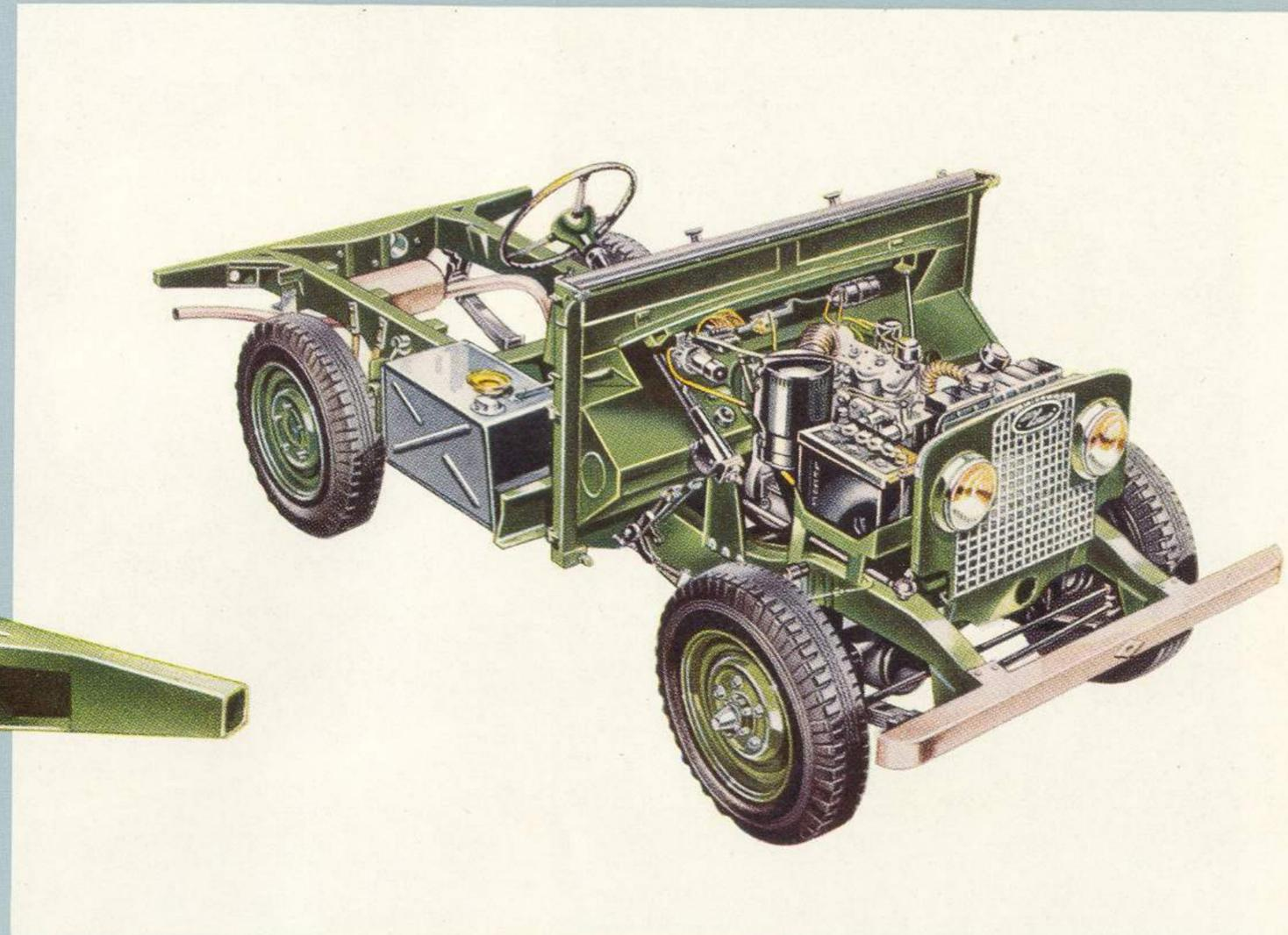
The layout of the engine compartment is compact yet the individual units are so placed that they are readily accessible for maintenance and adjustment.
