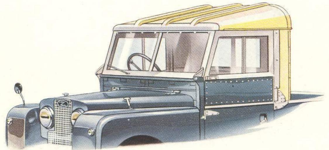
Truck type cabs are fitted as standard equipment on the long wheelbase model but can also be supplied as an optional extra on the 86 in. wheelbase vehicle. A tropical roof is available for this type of unit.
