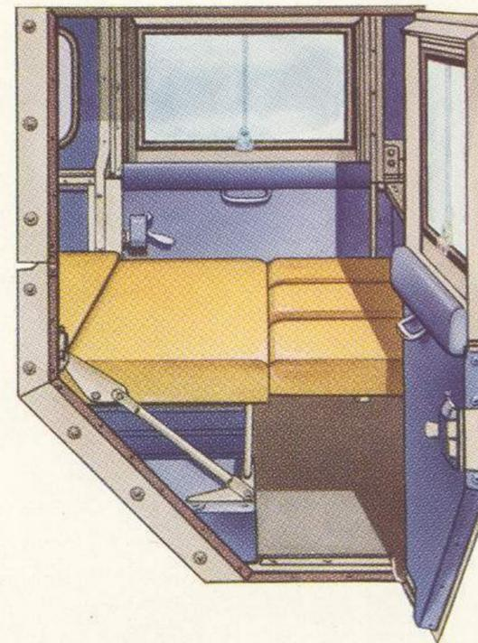
Additional seats mounted on the rear wheel boxes will carry four passengers, two on each side.
