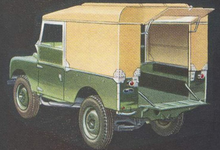
A wide rear door and folding step give easy access to the rear seats of the Land-Rover Station Wagon. The door is lockable.
