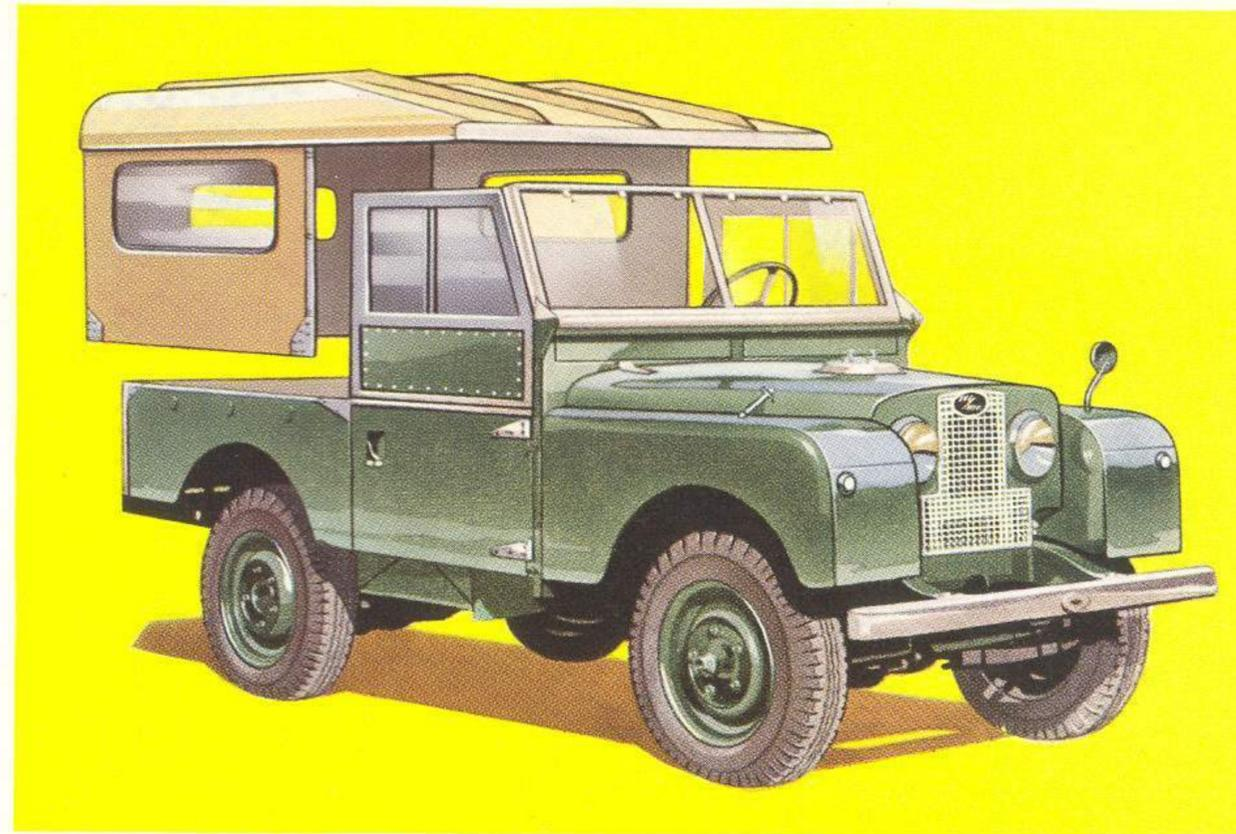
A de luxe cab is an optional extra on the 107 in. wheelbase Land-Rover. With trimmed door casings and carpets it affords a very high standard of comfort for driver and passengers.
