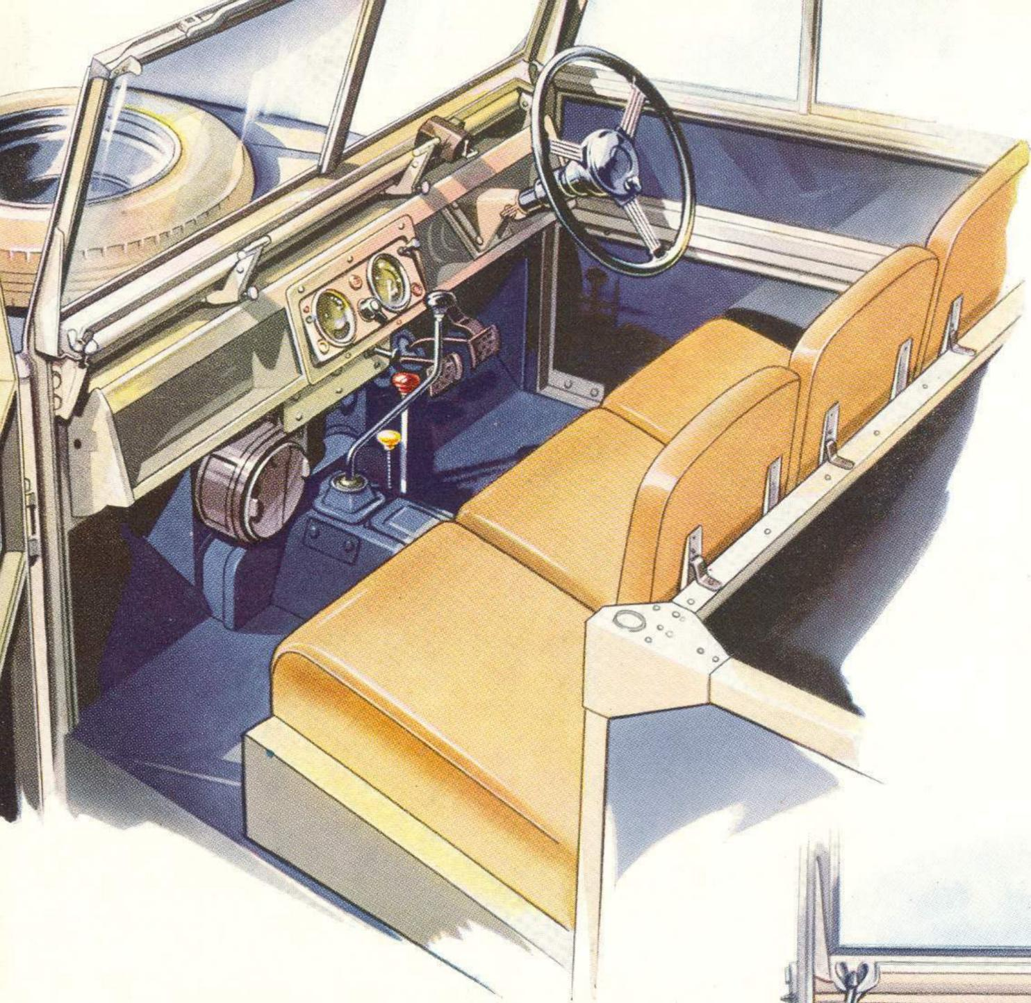
A recirculatory type of heater can be supplied as an optional extra. It fits neatly under the dash and operates efficiently to give ample warmth in the coldest weather. Attachments are provided for windscreen defrosting.
