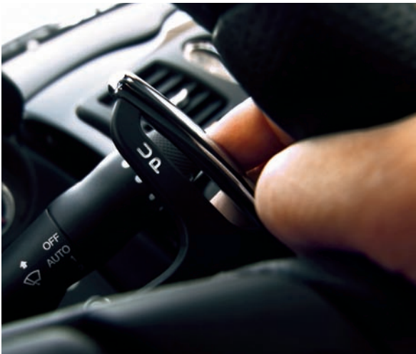
OPTIONAL PADDLE SHIFTERS MOUNTED ON COLUMN OF STEERING WHEEL.
