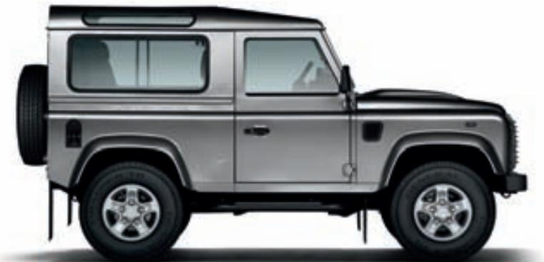
Defender (2007-Present) 2007 2.4 litre diesel engine, six-speed manual transmission and new interior introduced.
