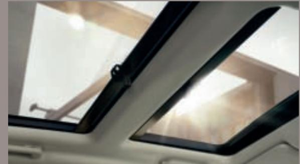
**PANORAMIC SUNROOF** The standard panoramic sunroof – with a fixed rear section and electric tilting/sliding front section – adds to the feeling of lightness and airiness within the cabin. The glass is specially formulated to filter the sun's infrared rays, providing light without unpleasant heat. Both sections also include a convenient blind.
