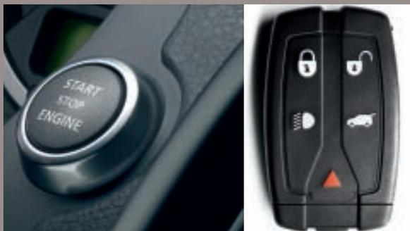
**REMOTE CONTROL AND START/STOP BUTTON** The remote control includes the following functions: locking and unlocking of the doors and tailgate, a 30 second courtesy headlight delay and activation of panic alarm. In order to start the car the remote has to be docked into the fascia and the correct procedure followed using the Start/Stop button.
