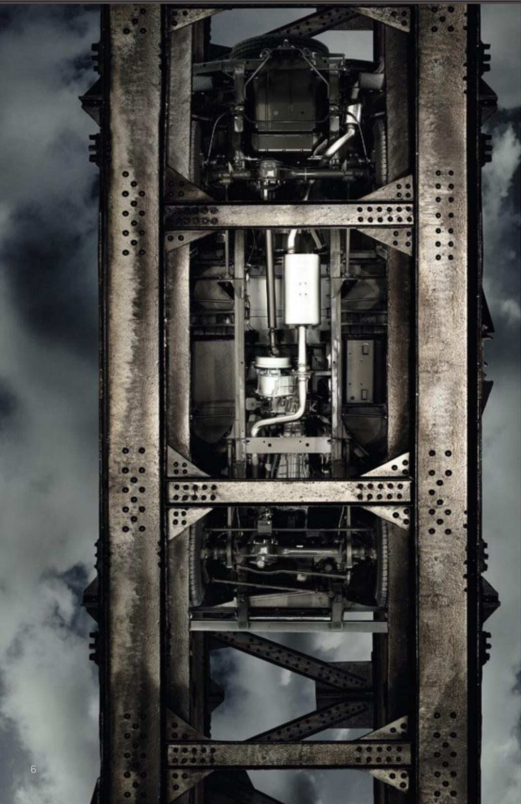
There are some things that'll never need improving. Defender's chassis is one of them. Immensely strong, it is probably the single most important component in the vehicle's design architecture and contributes to its strength, versatility, durability and capability. The box section, ladder frame design is far stronger than an open channel design and more adaptable than the unibody design favoured by many of its competitors.
