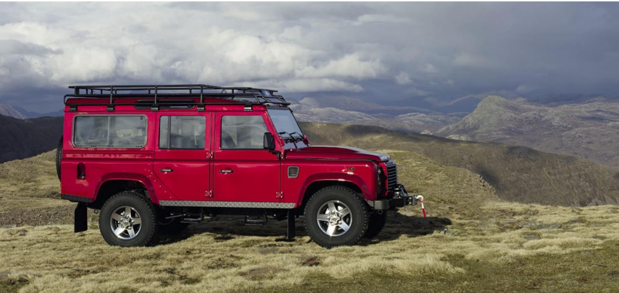
Defender 110SW shown above is accessorised with Expedition Roof Rack System, Black Wing Top Protectors, Black Chequer Plate Protection Kit, Front Mudflaps and Rear Mudflaps, 16 inch five-spoke alloy wheels – Dual Finish, Folding Side Steps and 9.5ti Electric Winch.
