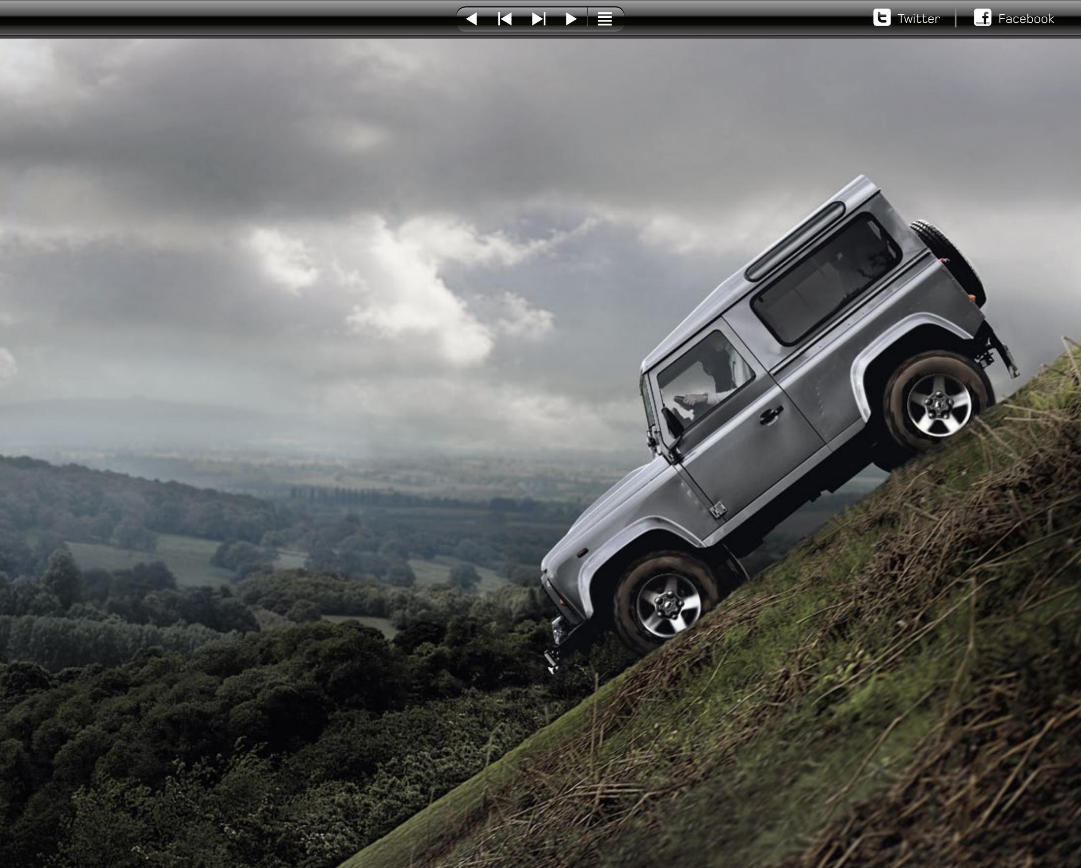
Unlike many of its competitors, Defender has permanent four-wheel drive with the centre differential distributing torque evenly between front and rear axles to give optimum performance on-road and off-road. What's more, the centre differential can be locked to help minimise wheel spin and maximise traction on slippery surfaces. And for even more grip and control off-road (not to mention on-road as well) Defender is available with an optional ABS system featuring traction control.
