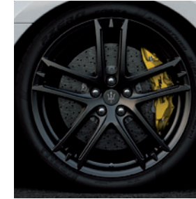
Brake calipers, painted Giallo Alloy wheels, 20" MC-Design Grafite Opaco (8,5J x 20" front; 10,5J x 20" rear)
