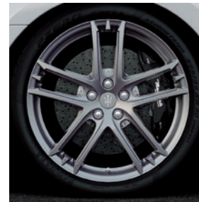
Brake calipers, painted Nero Alloy wheels, 20" MC-Design Titanio Lucido (8,5J x 20" front; 10,5J x 20" rear)
