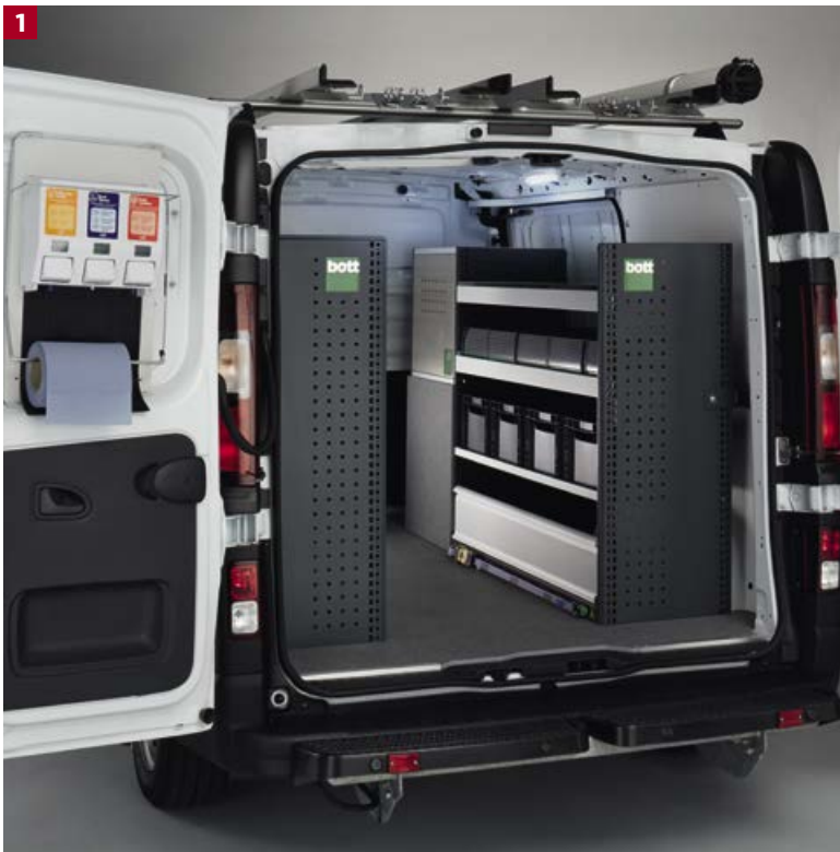
1. L1 H1 Vivaro fitted with a Bott vario vehicle racking system.
