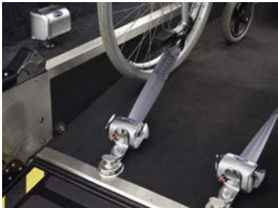
Secure wheelchair restraint system.
