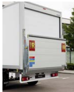
500kg capacity tail lift is optional at extra cost.
