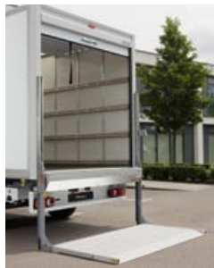
500kg capacity tail lift is optional at extra cost.
