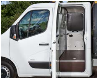
Utility cab option provides a secure storage space.
