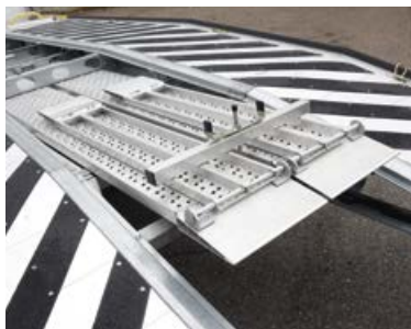
Lightweight aluminium loading ramps in stowed position.
