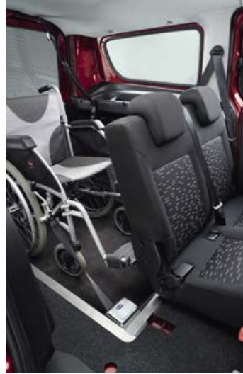
Lowered floor for wheelchair position.
