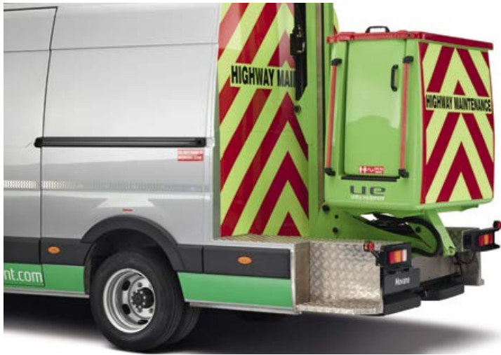
Protected rear basket position reduces overhang and kerbweight.
