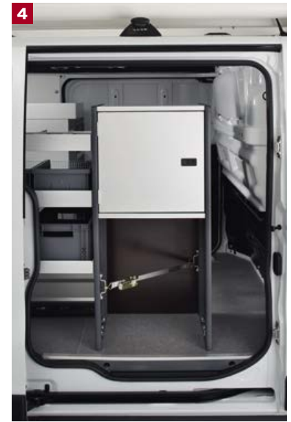
2-3-4. Vivaro L1 H1 featuring fixed shelves with dividers, cupboards, drawers and aluminium drop front.
