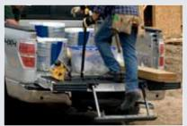
TAILGATE STEP is a classexclusive option that makes accessing the cargo box easy. Just raise the grab bar and flip down the skid-resistant step. Stows in the tailgate.
