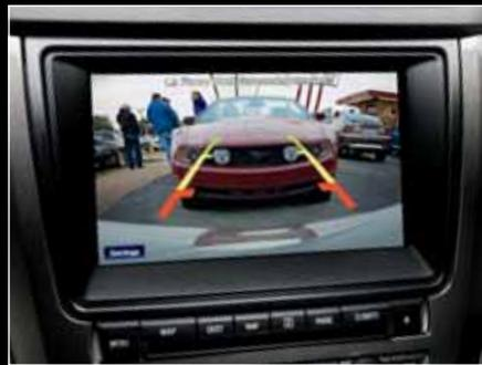
**REAR VIEW CAMERA** is an optional help. Shift into reverse – a full-color image from the spoiler-mounted camera appears in your rearview mirror or on the available navigation screen.
