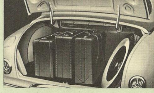
ROOM TO SPARE—For loads of luggage on the longest trip. Automatically illuminated compartment is safety-sealed against dust and water. The spare tire is at the right—convenient, yet out of the way.
