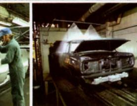
fenders and other front-end sheet metal stampings made of galvanized steel. And to help the sheet metal resist corrosion, each truck body is prepared for the primer coat by a
