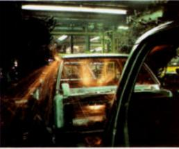
Dodge uses galvanized steel in many critical body areas to help protect against corrosion. For example, galvanized steel is used for the floor, inner side panels, wheelhousings, stake
