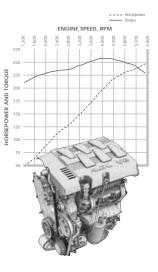
3.3-LITER OHV 12V V6 175 horsepower @ 5,000 rpm; 205 lb-ft of torque @ 4,000 rpm
