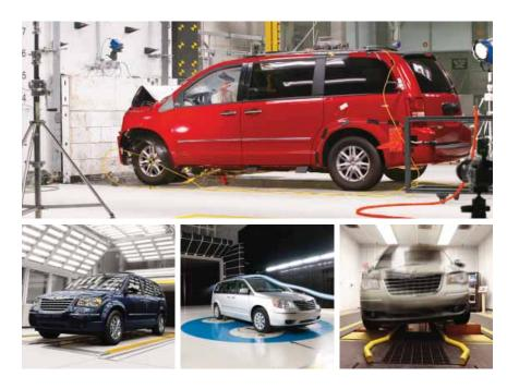
Top: Town & Country testing in action during a high-speed crash test. From left, functionality evaluations under extreme temperatures, improving aerodynamics with the help of a 100-mph wind tunnel, and working out NVH kinks on the four-post shaker.
