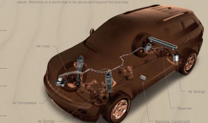
With an easy turn of a dial, your Grand Cherokee's traction control is adjusted to match the driving conditions facing 4WD you on the road ahead. Whether you're hills, available Selec-Terrain gives you the confidence to bravely meet all challenges. Five selectable settings of Grand Cherokee's powertrain, braking and suspension systems. Couple with the available and all-new four-corner Quadra-Lift, and you'll be at the forefront with Best-
