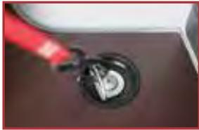
It's designed for convenience — and to help protect cargo. The standard load floor offers up to ten steel tie-down rings, each rated at 1,000 lb, to secure cargo; additional rings (in the walls and partitions) can total up to 17. Pre-cut holes in the available resin-finished wood load floor guarantee easy access to every ring.
