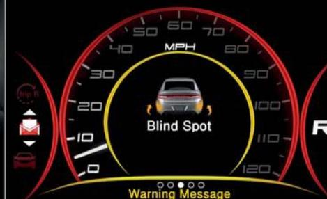
///// Available Blind Spot Monitoring (BSM)<sup>[2]</sup> Radar continually monitors rear vehicle blind zones on either side of the vehicle.\*
