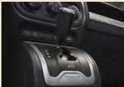
SIX-SPEED AUTOMATIC TRANSMISSION WITH AUTOSTICK: *Enjoy a smooth ride regardless of whether you're traveling over road or trail. This available six-speed PowerTech automatic transmission has a low first gear for quicker takeoffs and a tall top gear for relaxed highway cruising. A stepped shift schedule across all six gears is designed for optimal city fuel efficiency. The fact that the transmission fluid's fill-for-life design helps reduce maintenance costs just adds to the pride of ownership.*
