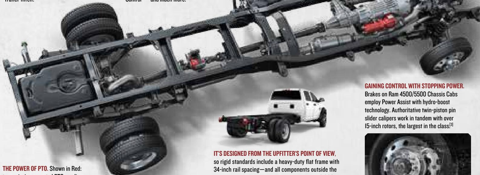
**THE POWER OF PTO.** Shown in Red: transmission-mounted PTO sending unit and split-shaft PTO element.
