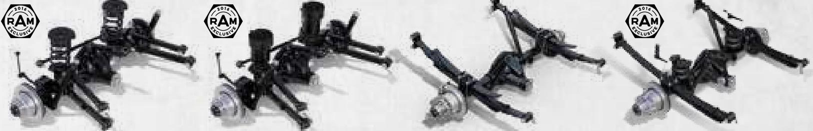
**2500: THE REAR FIVE-LINK COIL SPRING SUSPENSION.**<sup>[8]</sup> The five-link coil spring rear suspension, standard on Ram 2500, is revolutionary in the heavy-duty pickup segment. It's engineered to spec, providing outstanding ride/handling characteristics and beyond-dependable hauling and payload capability, irrespective of load.
