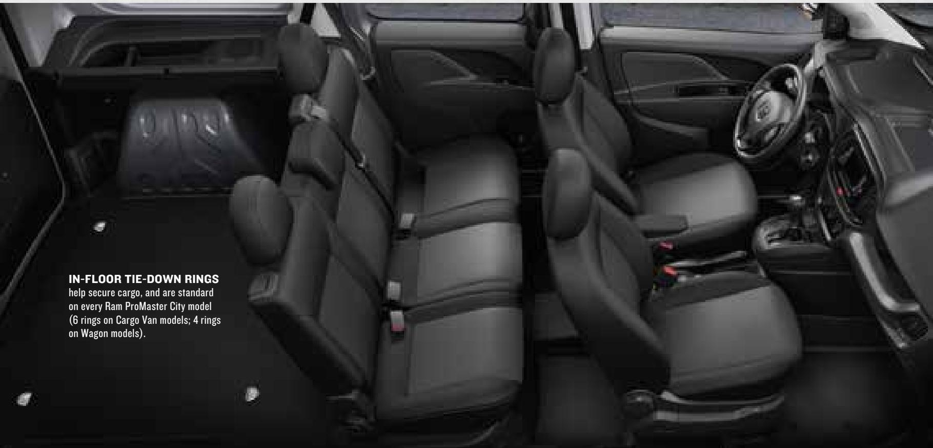
**IN-FLOOR TIE-DOWN RINGS** help secure cargo, and are standard on every Ram ProMaster City model (6 rings on Cargo Van models; 4 rings on Wagon models).
