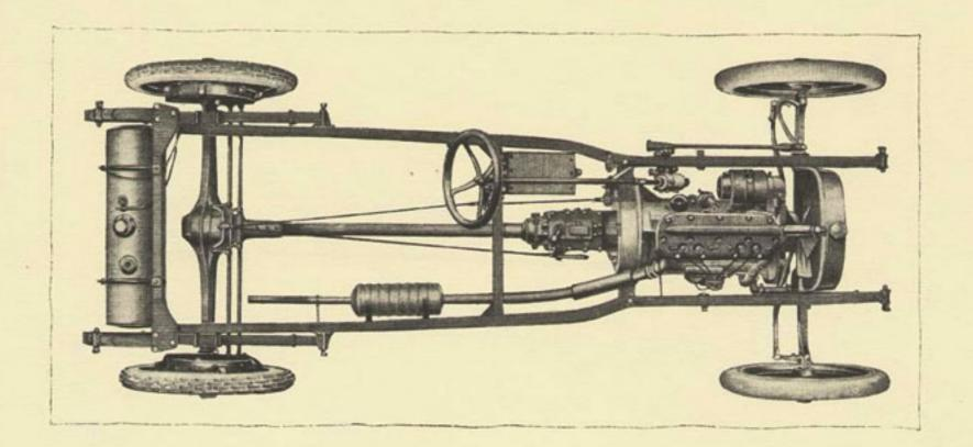
Transmission — Selective sliding gear type giving three speeds forward and reverse.
