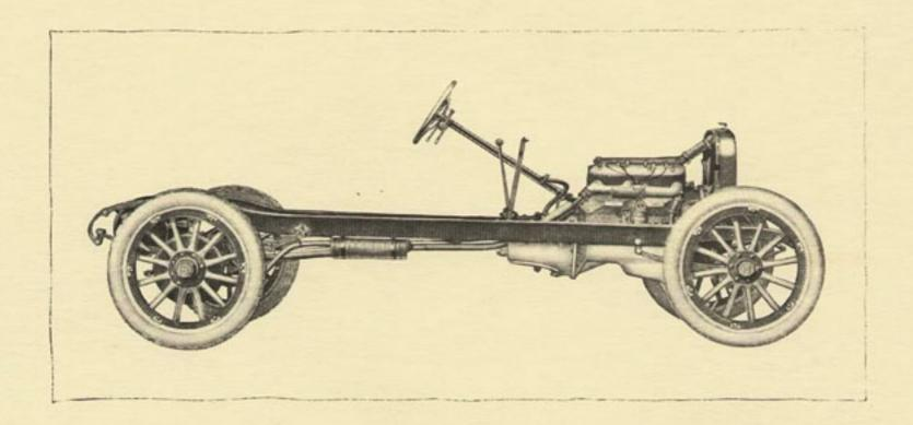
Engine—30-35 H. P. 3-point suspension unit power plant. Compression 64 pounds per square inch. 380 R. P. M. at 10 miles per hour on direct drive.
