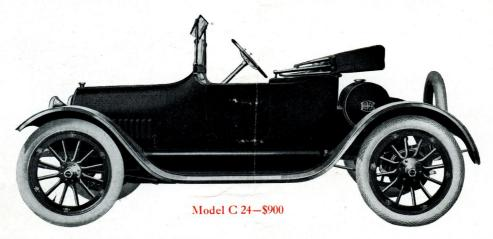
A comfortable roadster, with deep roomy seat, plenty of leg room, amply powered, easy to handle, economical in operation, 28 actual H. P., 106-inch wheel base,  $32x3\frac{1}{2}$  tires, anti-skid in rear, complete Delco equipped for starting and lighting, all electric lights, electric horn, license plate hangers, inside operating side curtains. In fact, up to the minute in every particular.
