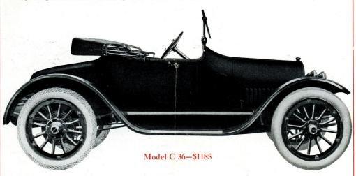
Richly appointed, and generally accredited the handsomest roadster of the year. Complete in every detail. 112-inch wheel base, 34x4 tires, anti-skid in rear, brake test 35 H. P., unit power plant, three-point suspension, twenty-gallon gasoline tank, extra deep cowl with instrument board, fully electric lighted, Delco system for starting and lighting. All appointments rich and refined.
