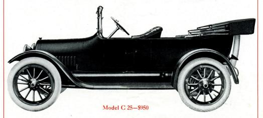
An ideal family vehicle at a price that places it within reach of anyone. Plenty of room for five and plenty of power for any load. Wheel base 106 inches,  $32x3\frac{1}{2}$  tires, anti-skid in rear, 28 brake test H. P., complete electric equipment, Delco system, new windshield, inside top curtains, and every other feature necessary to make it a car for the family.
