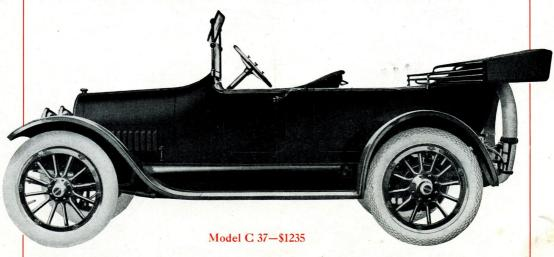
A beautiful streamline body, with graceful cowl; extra wide deep seats, advanced ideas in design and every detail making for utility, places this car at once in a class of its own. 35 actual brake test H. P., 34x4 tires, anti-skid in rear, wheel base 112 inches. Full Delco equipment for starting and lights. Inside curtains, new shield and every feature of notable excellence.
