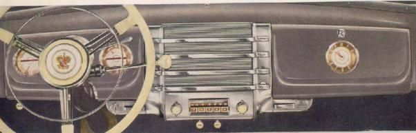
The handsome instrument panel of the SPECIAL puts the driving instruments right in the driver's line of vision. Lights, heater and accessories are controlled by switches that form extensions of the bars of the radio grill. To the right are the clock and fresh-air adjustment.
