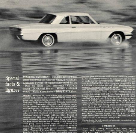
Automatic transmission is the divided torque type with approxi-
