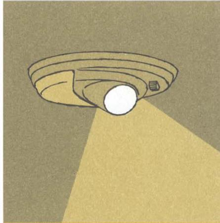
**DOME AND READING LAMP** . . . permits passenger to read or study maps at night without light disturbing driver. Concentrated spot beam is supplied by lamp mounted on interior ceiling. It swings a full 360° for flexible positioning . . . has independent switch. (F)
