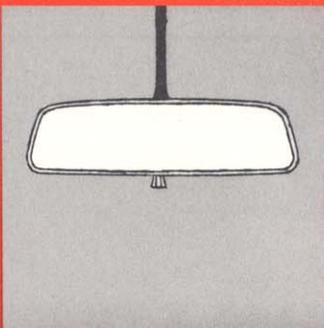
**INSIDE NON-GLARE REAR-VIEW MIRROR**... has special finger tab to permit easy adjustment to non-glare or nighttime driving position. Mirror position indicated by tab. **(FD)**
