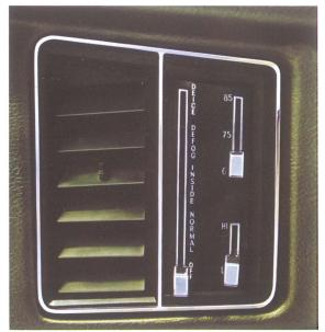
Automatic Temperature Control Air Conditioning. Available on Catalina, Executive, Bonneville and Grand Prix models. Select a temperature and forget it. Built-in sensors automatically maintain interior at desired pre-set comfort level year 'round. Dehumidifies, too. New, convenient lever controls.
