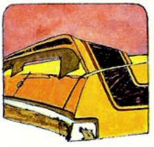
SPOILERS! Stylish, molded fiberglass rear deck spoiler acts with the front spoiler which is tucked under the bumper of every GSX. They help keep the front and rear end down for improved traction and handling.
