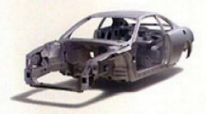
Safety cage construction is designed to help preserve the integrity of the passenger compartment during impact.
