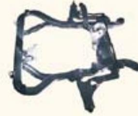
**Vibration-isolating subframe.** Since we assumed you wanted a smooth, comfortable ride, eliminating vibration was our top priority. So our engineers designed a special subframe with six mounting points (most cars have four) to help keep engine and transmission vibrations where they belong—out of the passenger cabin.
