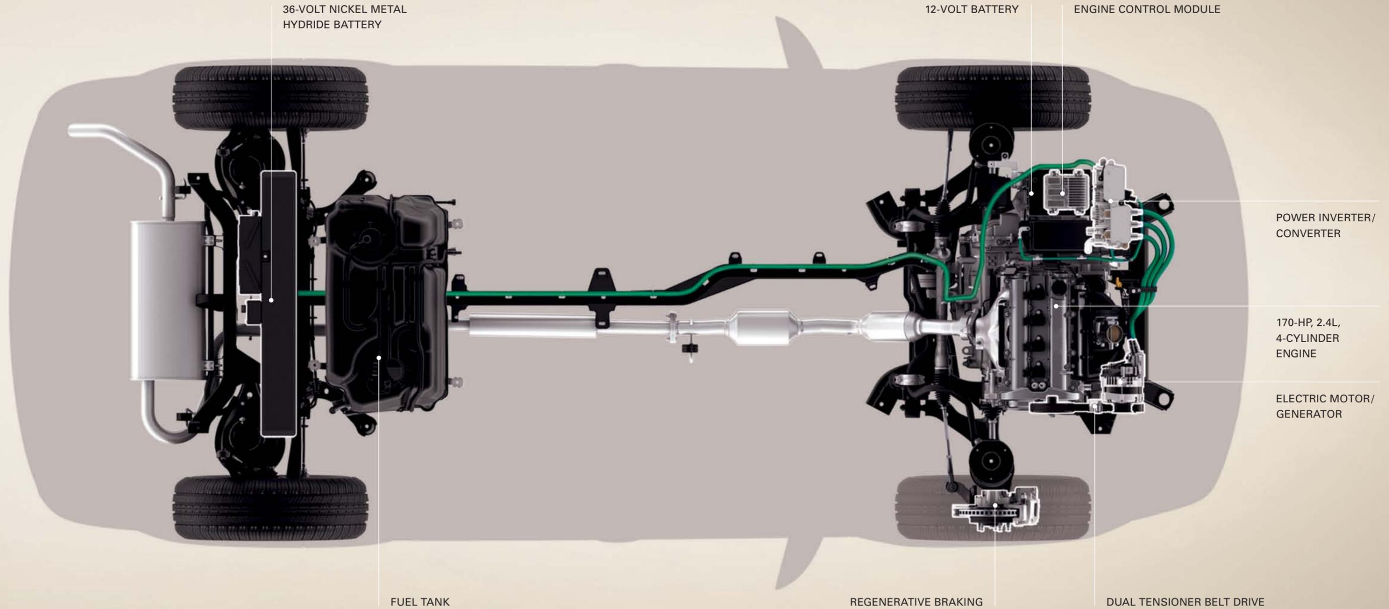
AT A COMPLETE STOP, the VUE Green Line's 36-volt battery powers the vehicle accessories, allowing the gas engine to shut off and save fuel.\*
