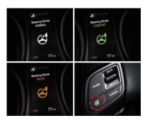
**SMARTER STEERING** Santa Fe Sport is the first CUV to feature Driver Selectable Steering Modes, which allow you to choose your preferred mode of power steering – Comfort, Normal or Sport – using a button on the steering wheel for a more customized feel behind the wheel.
