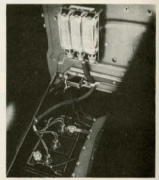
matic Battery Filler on the current series cars, although it can be installed and is available for all previous models.
