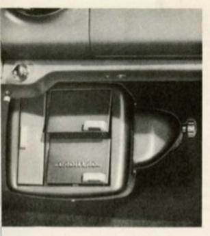
to the driver. The switch has six positions: high, medium and low speeds for direct heating, and high, medium and low speeds for indirect heating. The switch is an attractive plastic moulding and is illuminated. It is connected to the ignition switch to prevent its being left on when leaving the car.
