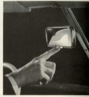
of the mirror snaps the mirror into the "Nite" position, when light is reflected from the front surface of the mirror and assures glareproof rear vision at night. The mirror back is gold-surfaced instead of silver for soft, clear reflection.
