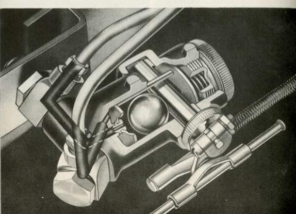
Its operation is shown graphically in the three-position sketch to the right. In the first sketch, showing the clutch engaged, and the car on a level, the valve "B" is held away from its seat "C", permitting free passage of the brake fluid from the brakes to the master cylinder, regardless of the position of ball "A".
