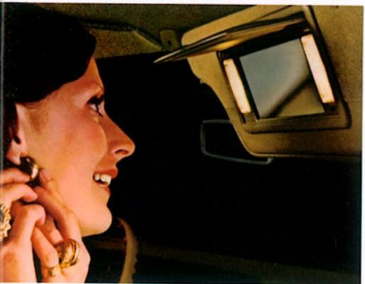
Lighted Vanity Mirror. Available on sun visors for both driver and passenger sides (passenger side only on Convertible). Raising the protective cover turns on lamps, one on each side of the mirror. Selector switch for high- or low-intensity light. Tilted, makes an excellent map light. Right-hand version is standard on Talisman.
