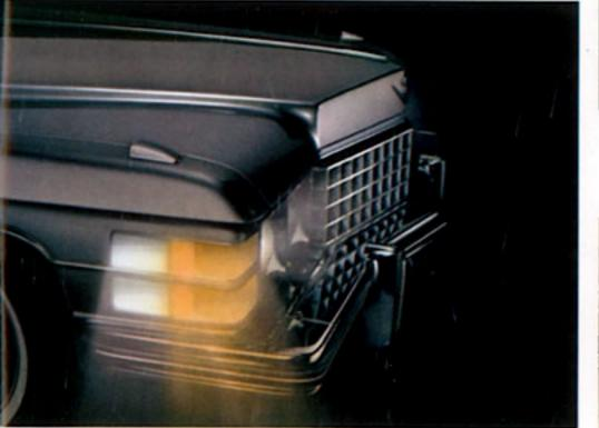
Cornering Lights. For added convenience when driving at night, these lamps project a beam of light from the side of the car to illuminate the roadside and road signs when making a left or right turn. They're located on the side of each front fender and blend beautifully with the front end design of every 1974 Cadillac. The directional turn signal lever will activate them whenever the headlamp switch is on.
