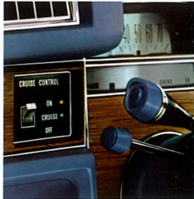
Cruise Control. A touch of this control at the tip of the directional turn signal lever allows you to maintain a selected speed without using the accelerator pedal. Unit automatically disengages when you apply brakes or turn off ignition.
