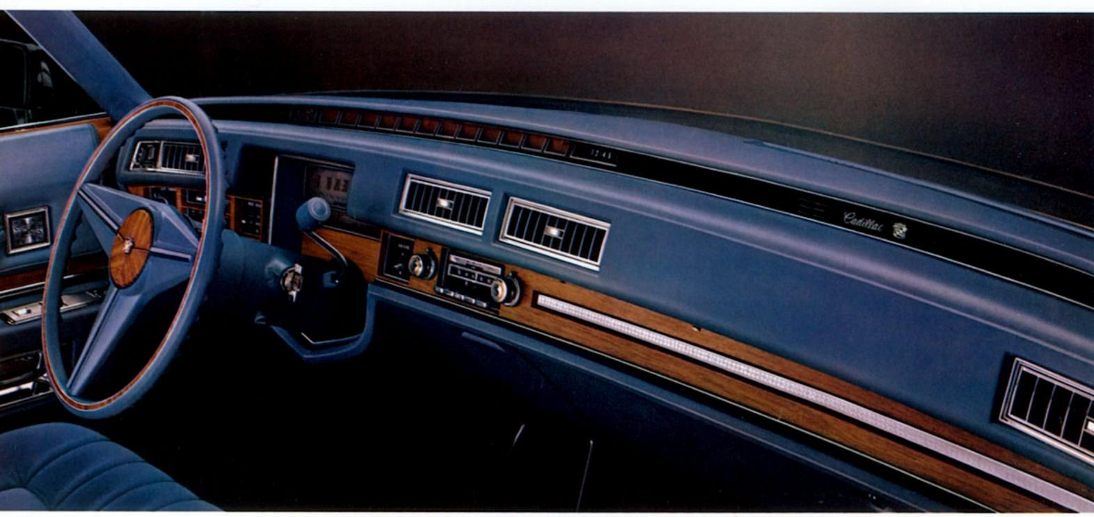
New Instrument Panel. A new concept in instrument panel design has given a definite lap-of-luxury look to every 1974 Cadillac, while attaining an extremely high degree of organization. The fuel gauge and numerous warning lights have been grouped into a band across the upper portion of the instrument panel. This year's standard timepiece, a precision digital clock, is in the information band as well, in the exact center of the car. The more immediate driving functions (speedometer,
