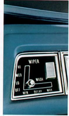
for 1974. Adjustable delayed action for light rain (up to 10-second intervals between wipes).
