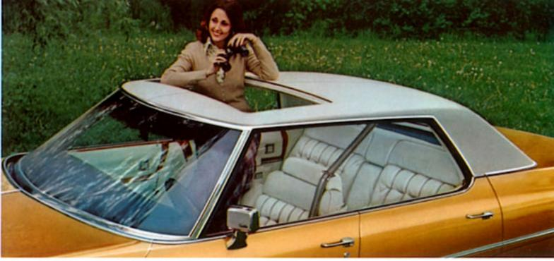
Electrically Operated Sunroof. Simply flick a control switch on the instrument panel, and a roof panel slides open overhead to let in the sunshine. It is available on the Fleetwood Brougham, on the Eldorado Coupe with vinyl roof and DeVilles with vinyl roofs, also Calais when vinyl roof is ordered.
