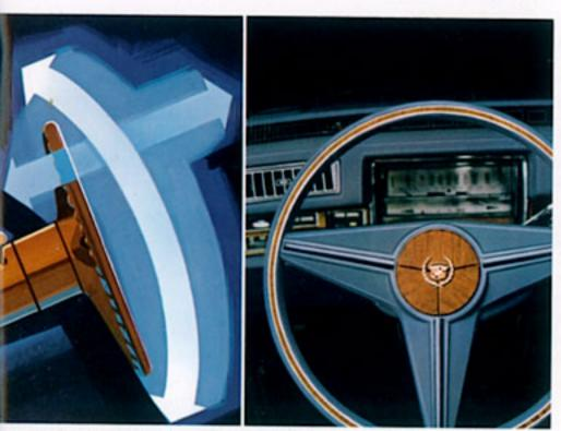
Tilt and Telescope Wheel. This adjustable steering wheel can be tilted up or down and moved backward or forward to accommodate driver's height and reach. Swings up for easy entry and exit.
