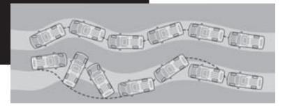
Without StabiliTrak, a simple lateral skid can quickly turn into a dangerous spin, as shown in the lower illustration. StabiliTrak helps to avoid spins by bringing lateral skids to an early end. It's a major contributor to driver control and safety.
