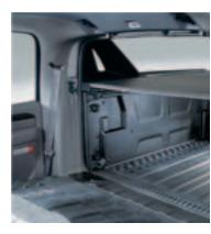
With the rear seat and Midgate folded down and the three-piece tonneau cover in place, Escalade EXT offers an immense 2690 L (95 cu. ft.) cargo area that's 2.4 m (8 ft.) long.
