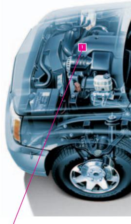
345 hp Vortec 6000 V8. The Corvette-inspired LQ9 powerplant includes such features as computer-controlled sequential fuel injection, a high-flow intake manifold and low-restriction intake and exhaust ports. A high 10.1:1 compression ratio and lightweight aluminum cylinder heads contribute to excellent performance.
