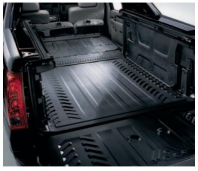
The sides of the cargo box are protected by a tough, scratch-resistant liner. A non-skid rubber composite material on the bed floor helps to keep cargo from shifting when you're on the move.
