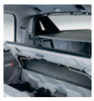
To create additional space for larger cargo items, simply flip the rear seat forward, remove the glass window panel and fold down the Midgate.
