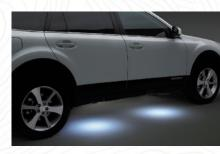
**Puddle Lights.** L.E.D. lights activate when vehicle doors are unlocked using the keyless entry. A soft glow illuminates the ground, aiding entry and exit of the vehicle.
