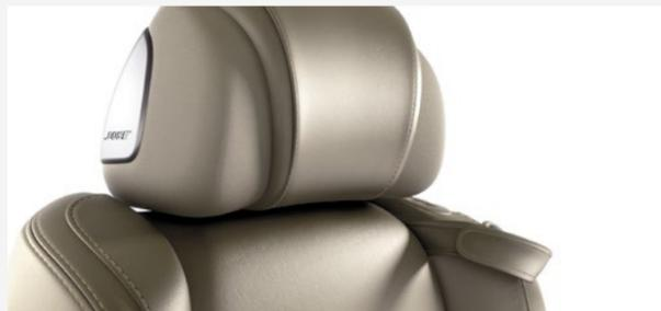
**THE SUPPORT YOU NEED** In certain rear-end collisions, the Front-seat Active Head Restraints found on the Q60 Convertible can move forward to help cushion the head to help reduce whiplash-type injuries.
