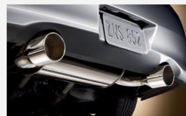
**SPORT MUFFLER** The polished, stainless steel muffler showcases a deeper, throaty exhaust tone. Larger-diameter exhaust tips help let it breathe and the muffler is fabricated with TIG welds not only for appearance but for strength and longer life.
