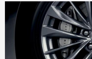
**SPORT BRAKES<sup>1</sup>** Aluminum 4-piston opposed front calipers with ventilated discs and 2-piston opposed rear calipers with ventilated discs provide great stopping force from both sides of the rotor at the same time for better bite, more friction and direct feel.
