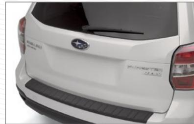
**Rear Bumper Cover.** Helps protect the upper surface of painted rear bumper from scratches and dings.
